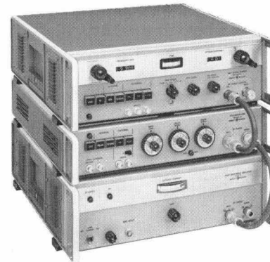
Fig. 13. Combination of new Model 8614A Signal Generator, 8714A Modulator, and 489A TWT Amplifier comprise high-performance signal generator with output of 1 watt.
